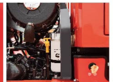
• Easy oil-water separator replacement and maintenance • Easy engine oil adding and check
